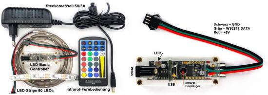
Special circuit for controlling WS2812 strips via infrared remote control. The LED box includes the LED-Basic controller, an LED strip with 60 LEDs, infrared remote control and power supply. Ideal for apartment effect lighting. Using the LDR, the strip brightness can be adjusted dependent on ambient light. EEPROM with 8 memory locations. Terminal display and error output via USB. Power supply via 5v/3a adapter.
