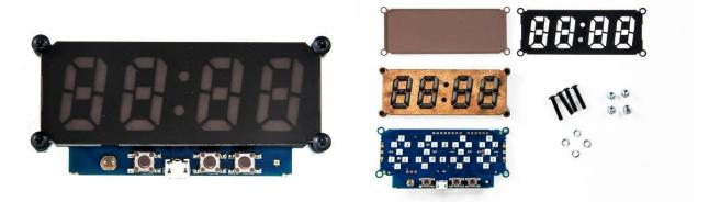
Kit for a 4-digit 7-segment clock with coloured numerals consisting of SK6812 mini LEDs. Terminal display and error output via USB. The board includes an integrated real-time clock with support battery. 3 keys or input pins, 3 output pins for switching signals, LDR and loudspeakers. Has suitable connection for optional temperature sensor DS18B20. Power supply via USB port. In addition to the 30 hardwired LEDs, the output (Dout) can be used to control up to 256 LEDs.
