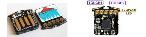
Mini USB stick with LED-Basic programming capability. 5 Mini-APA102 LEDs, 2 touch sensors. EEPROM with 16 memory locations. Output via terminal. Display and error output via USB. USB power supply.
